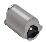
Model: WM-2000C-FHSX Physical: Nickel plated, hardened Zinc-Alloy Operation Environment: Temperatures: -4°F to 158°F (-20°C to 70°C); Humidity: 20% to 97% Weight: 93.4g Power: None, power supplied by key Audit Capacity: 100 units blocked keys, 60 lock events Hardware Feature: Lock body rated IP68, drill resistant, attack resistant torque break, tamper resistant security features, no keyway to pick Swing Direction: LH & RH
